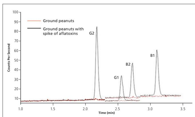
Figure 2. Overlaid SIM chromatograms of [M+H]<sup>+</sup> ions of aflatoxins B1, B2, G1 in ground peanuts spiked at 5 ppb level with aflatoxin G2 used as internal standard (spiked at a concentration of 20 ppb). A control sample of ground peanuts with no spike of aflatoxins is also shown
