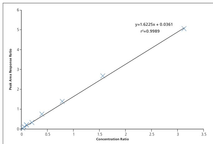
Figure 1. Calibration curve for aflatoxin B1 (0.48-63 ng/mL) using aflatoxin G2 as internal standard (20 ng/mL).
