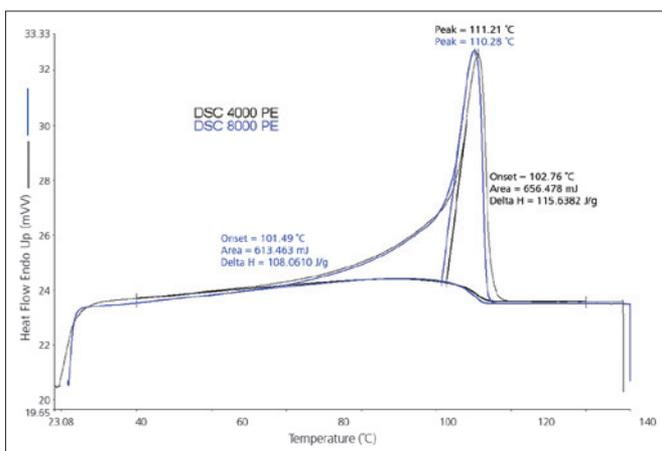
Figure 1. DSC curves for polyethylene acquired using a DSC 4000 and a DSC 8000.
