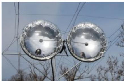
A normal concentrator cell is consist of lens which help focusing sun on perfect spot of cell, assembly of solar cell, device to waste of extra heat, wires for connectivity etc. These units are capable of combining with other units of different shapes and sizes to form bigger modules. Concentrator cells best works in direct sunlight, dry climates. Tracking devices must be used with these types of cells so that they can manage to keep their direction towards sun.
