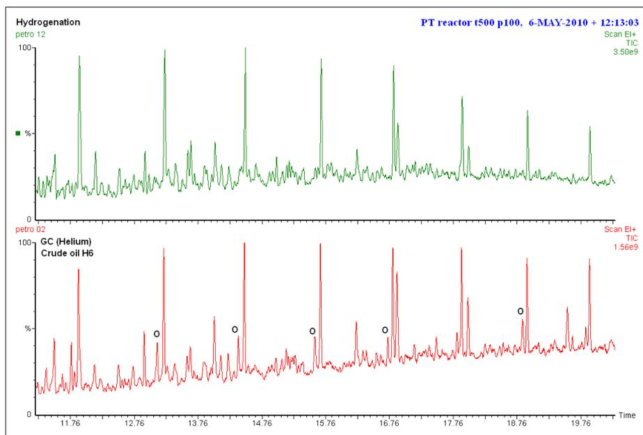
Figure 2. Expanded pyrograms of crude oil in He with olefins marked "O" (bottom), and H<sub>2</sub> (top).
