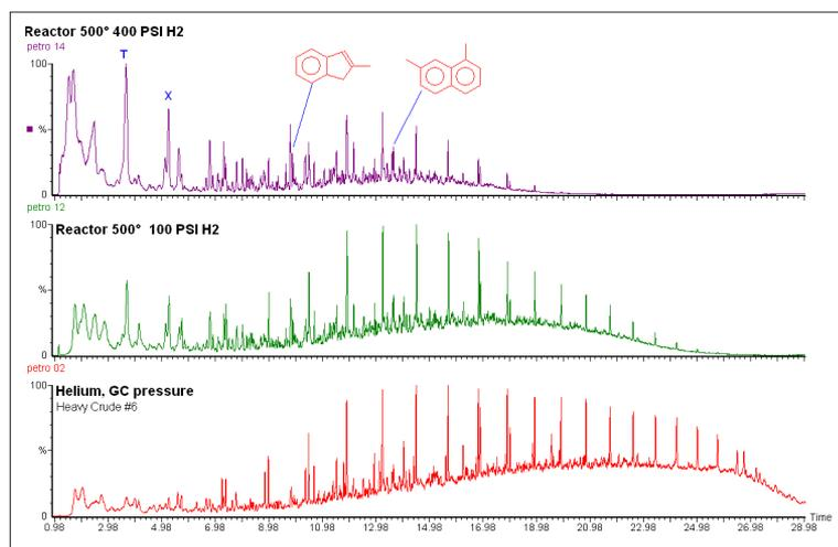
Figure 1. Py-GC of crude oil (bottom), at 100 PSI Hydrogen (center) and at 400 PSI (top)
