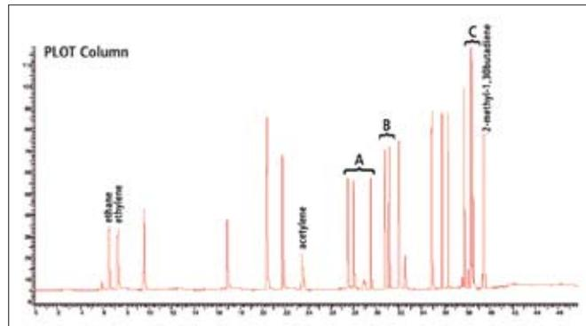
Figure 18. Critical separations on the alumina PLOT column.
