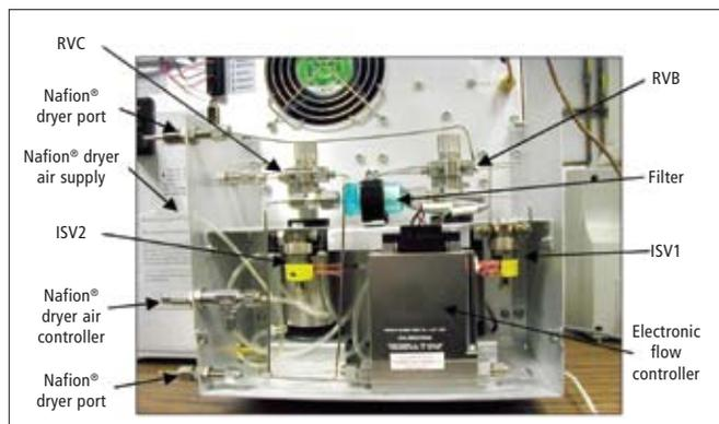
Figure 10. Cover removed from online sampling accessory showing key components.
