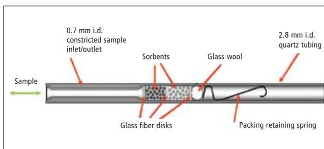
Figure 4. Internal geometry of the PerkinElmer Air Toxics Trap.
