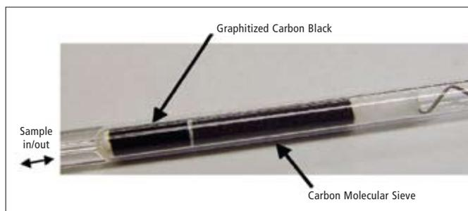
Figure 3. Photograph of the PerkinElmer Air Toxics Trap.
