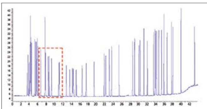
Figure 14. 10-ppb standard mixture chromatographed with effluent from methyl silicone column directed to FID1.
