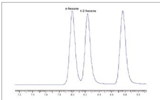
Figure 23. Critical separation 'D' – minimal baseline disturbance.
