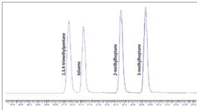
Figure 24. Critical separation 'E' – toluene reference peak well resolved.
