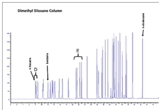
Figure 19. Critical separations on the dimethyl siloxane column.
