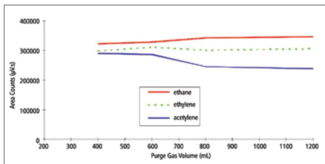
Figure 5. C<sub>2</sub> hydrocarbons recovery vs. sample gas volume (16-19 ng per compound).
