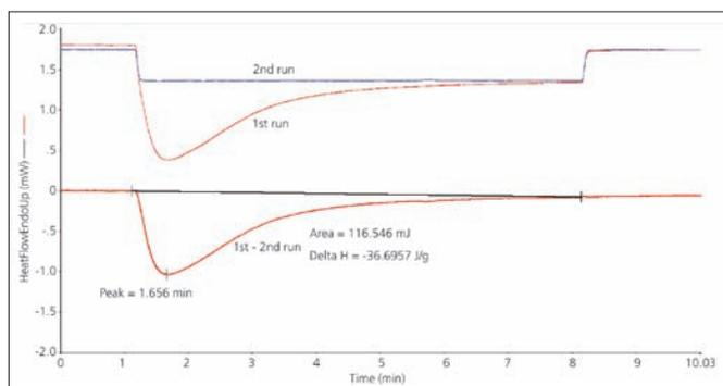
Figure 5. UV curing data process for the dental resin sample.
