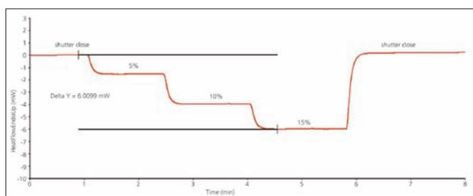
Figure 4. Light intensity determination by graphite disks.
