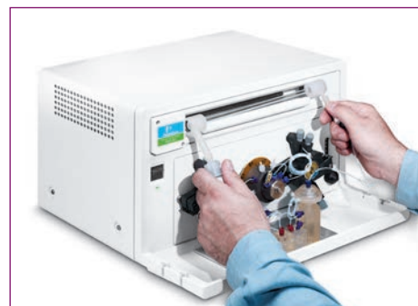
Easy interchange of FIMS absorption cell.
