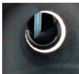
Figure 2. TubeView furnace camera on PerkinElmer's PinAAcle 900H, showing the optimized sampler tip depth inside the tube.
