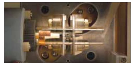
Figure 2. Torch-box of an Optima 8300 Flat Plate plasma technology.
