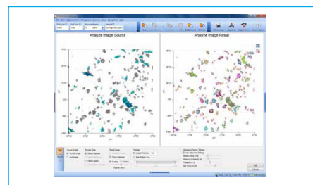
Figure 3: The Analyze Image software routine detects the particles in Product 1.
