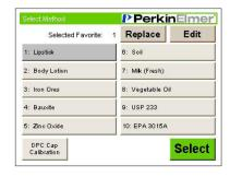
by a PowerPC™ CPU, delivers user-friendly tools for reaction control, data analysis, and storage of digestion data and user methods. The software comes preinstalled with a number of sample methods covering a wide range of digestion conditions – and the system accommodates any of the additional methods you create and come to rely on.
