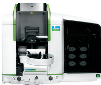
Figure 1. PerkinElmer PinAAcle 900T atomic absorption spectrophotometer.
