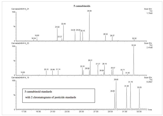
Figure 4. Pesticide elution times relative to cannabinoids.
