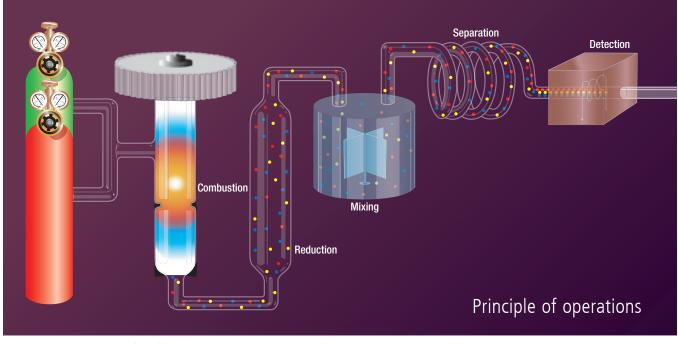
Figure 1. 2400 Series II CHNS/O Schematic.
